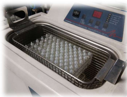
Figure 1: High throughput bar adsorptive microextraction (HT-BA \mu E) device operating under ultrasonic bath for the simultaneous microextraction of 100 samples.
